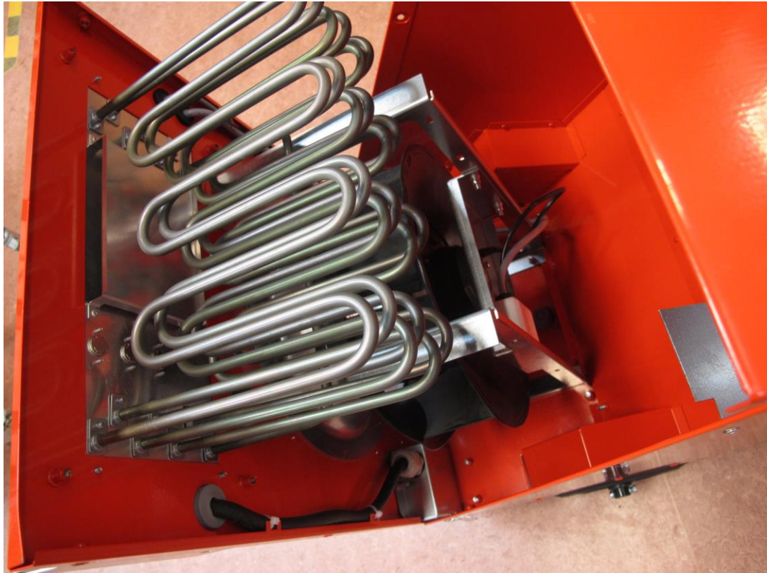
Figure 5. Fan and heating elements inside DT90.
