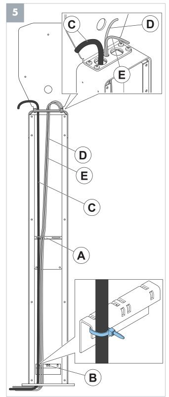
**Note**: Thread the cables (C, E and D) through the hole in the bracket (A). Use a zip tie to attach the cables to the bracket (B). Ethernet cable (E) and control cable (D) are optional.
