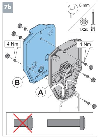
Note: Thread the cables through CS bracket (A) before you attach the bracket to the pole mount fixture and CS bracket (B).
