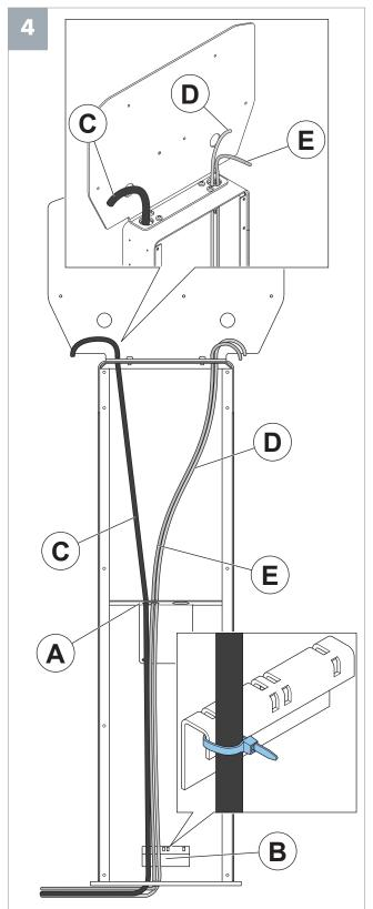
Note: Thread the cables (C, E and D) through the hole in the bracket (A). Use a zip tie to attach the cables to the bracket (B). Ethernet cable (E) and control cable (D) are optional.
