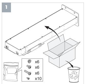
**Note**: The short screws are for single CS installation and the longs screws are for double CS installation.
