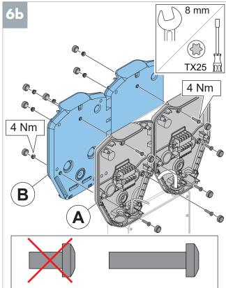
**Note**: Thread the cables through the double CS bracket (A) before you attach the bracket to the base and double CS bracket (B).
