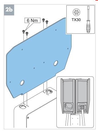
**Note**: Only when you plan to install two double CS units.
