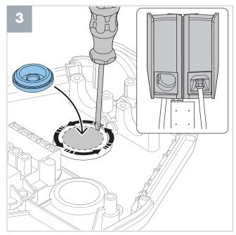
**Note**: Only if you install several CS on the ground stand. Do this on installation brackets of the charging stations. Use a cable grommet to seal the hole to the steelplate.
