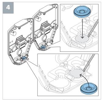
**Note**: Take notice of the position of the holes. It is possible to use a double installation bracket - EPIBD (GARO art. no 354214) or 2 singel installation brackets - EPIBS (GARO art. no 354213).
