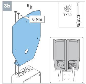
Note: Only when you plan to install two CS units.
