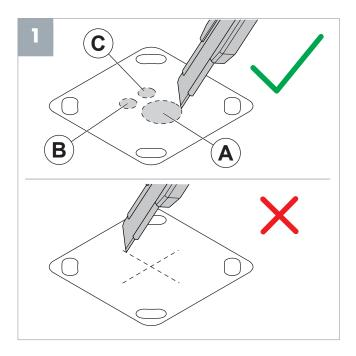
**Note**: A - Hole for the power cable. (Holes for an ethernet cable (C) and a control cable (B) are optional.)
