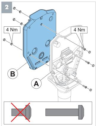
**Note**: Thread the cables through CS bracket (A) before you attach the bracket to the pole mount fixture and CS bracket (B).
