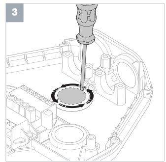
**Note**: Only if you install two CS on the pole mount fixture. Do this on installation brackets of the charging stations. Use a cable grommet to seal the hole to the steelplate.
