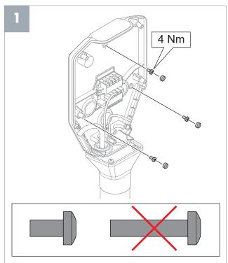
**Note**: A second CS can be installed on the back of the mounting plate of the pole mount fixture. In that case the long screws must be used.
