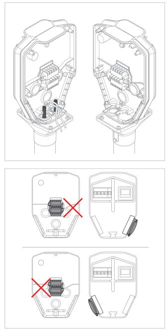
**Note**: For outlet versions only: Do not pinch the power cable wires. Do not route the wires on the same side of the connection terminal as the outlet.
