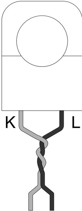
Wires -L are recommended to be light-twisted as pairs, to reduce induced disturbances.
