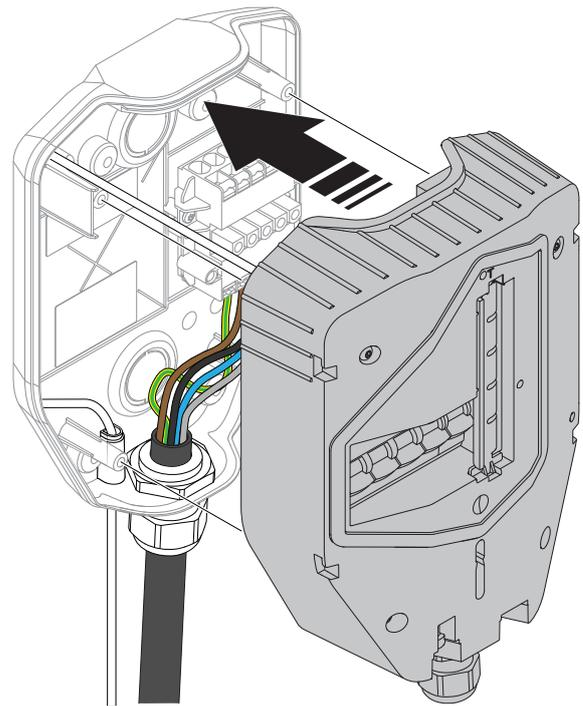
3. Use a Torx TX20 and tighten the 4 screws until the charging unit is tight against the installation bracket (max. 2,9 Nm).
