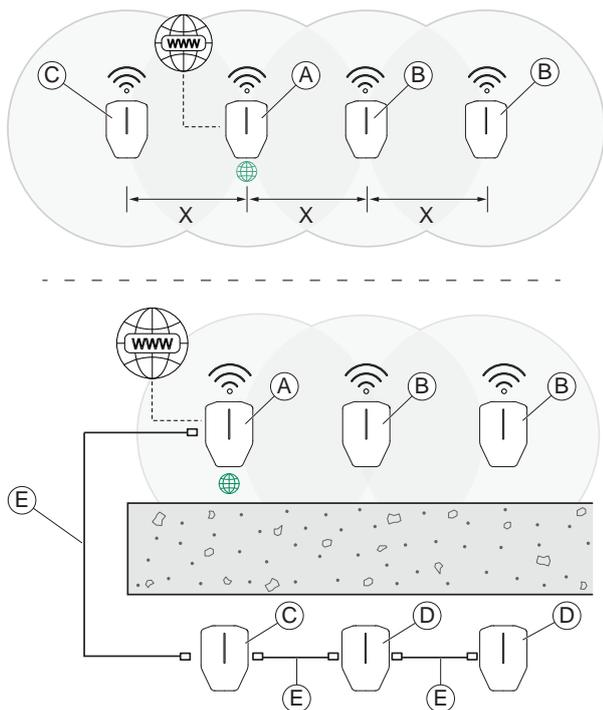
**Scenario 1:** If the distance (X) between the charging stations is short and there are no radio obstacles, it is possible to use a mesh Wi-Fi connection between the connection master charging station (A), and the other charging stations (B and C). However, it is always preferable to use an ethernet cable.
