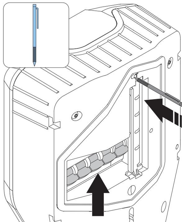
4. After the light goes off, release the button and the circuit breaker can be re closed. Refer to [5.5 To do a reset after a minor ground fault, page 78](#).
