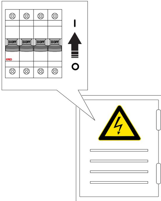
c. Wait for the charging unit to start. This takes up to 90 seconds and is shown with a green light indication given that the all-pole breaker is on, (else red).
