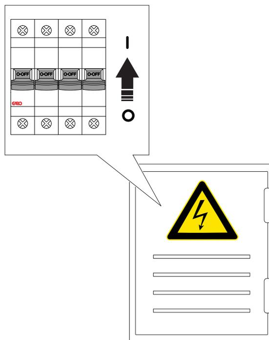
4. After the power is switched on, the Charging Station will startup. This can take up to 90 seconds. Progress is indicated by red LED-segments on the indication light. A fixed green light indicates when the charging station is ready given that the all-pole
