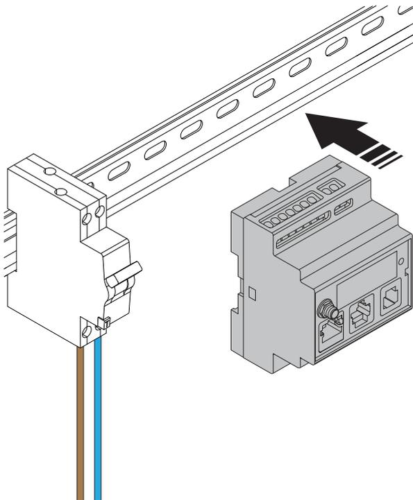
5. Dismantle the wires and connect the load interface to the 230V AC. Refer to the electrical schedule for all electrical connections.
