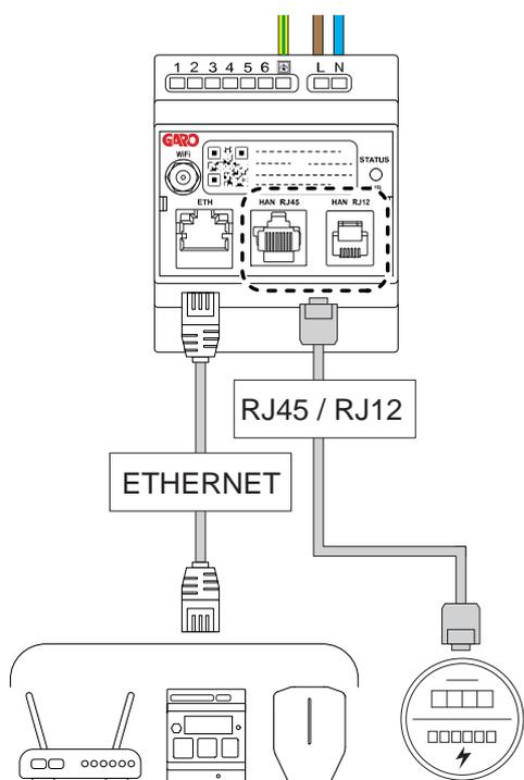
14. It is always recommended to connect an antenna even if a Wi-Fi or a mesh Wi-Fi is not used.
