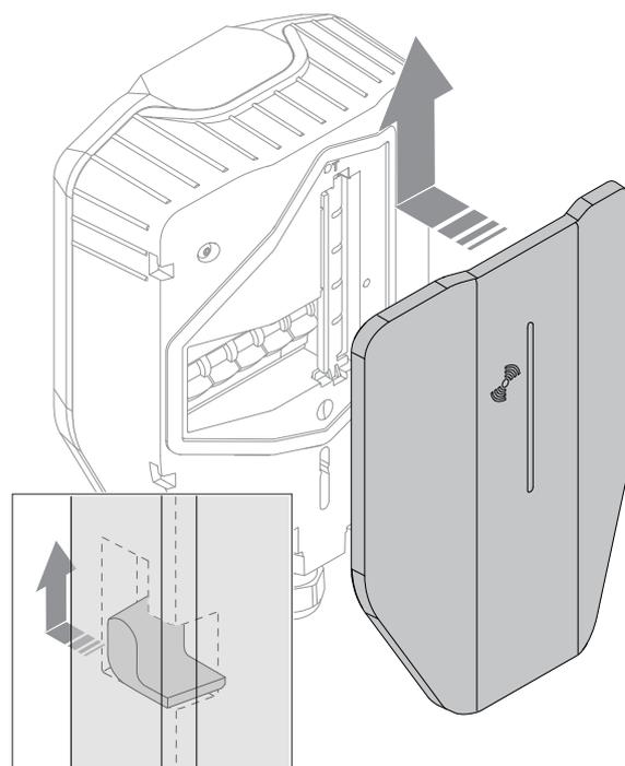
2. Use a Torx screwdriver to lock the front cover at the bottom of the charging unit. Tighten the screw with a maximum of 2 Nm.
