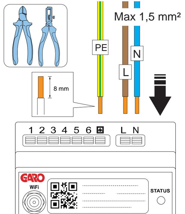
6. Connect the load interface to the protection device.
