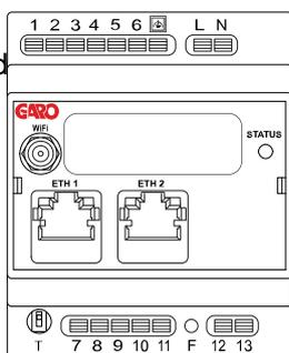
This is a general instruction of the load interface installation. The load interface is intended to act as an interface to the power and current meters as input to the DLM system of GARO Entity charging stations. The procedure differs between different installations and can also differ due to national regulations. The load interface unit is designed for DIN rail mounting. Two different load interface units are available at GARO: GARO Entity Balance basic and GARO Entity Balance advanced.
