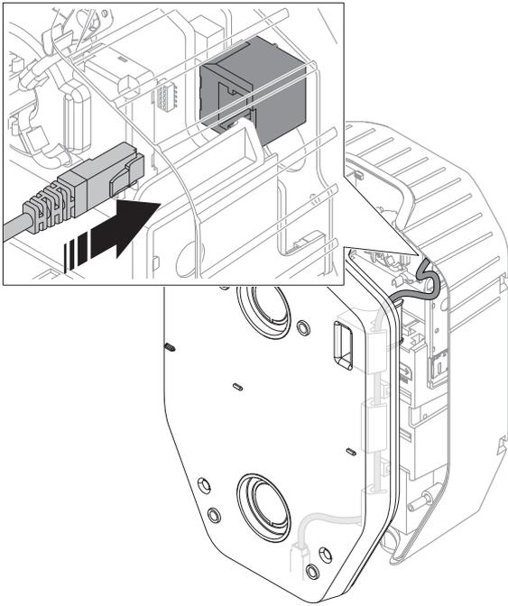
2. Attach the charging unit to the installation bracket. Press equally on the charging unit with both hands.
