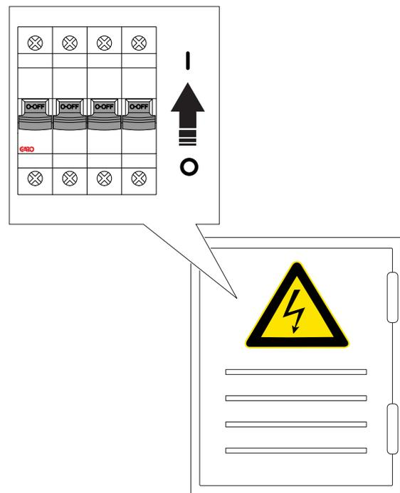
5. Do a check of the voltage and phase sequence in the installation bracket terminal. Make sure that the voltage and phase sequence matches the planned setup.
