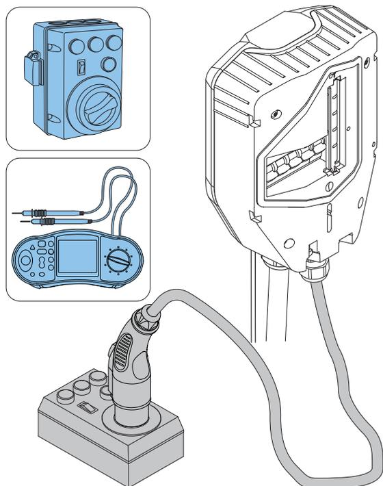
11. If necessary, reset the all-pole circuit breaker. Refer to [5.5 To do a reset after a minor ground fault, page 78](#).
