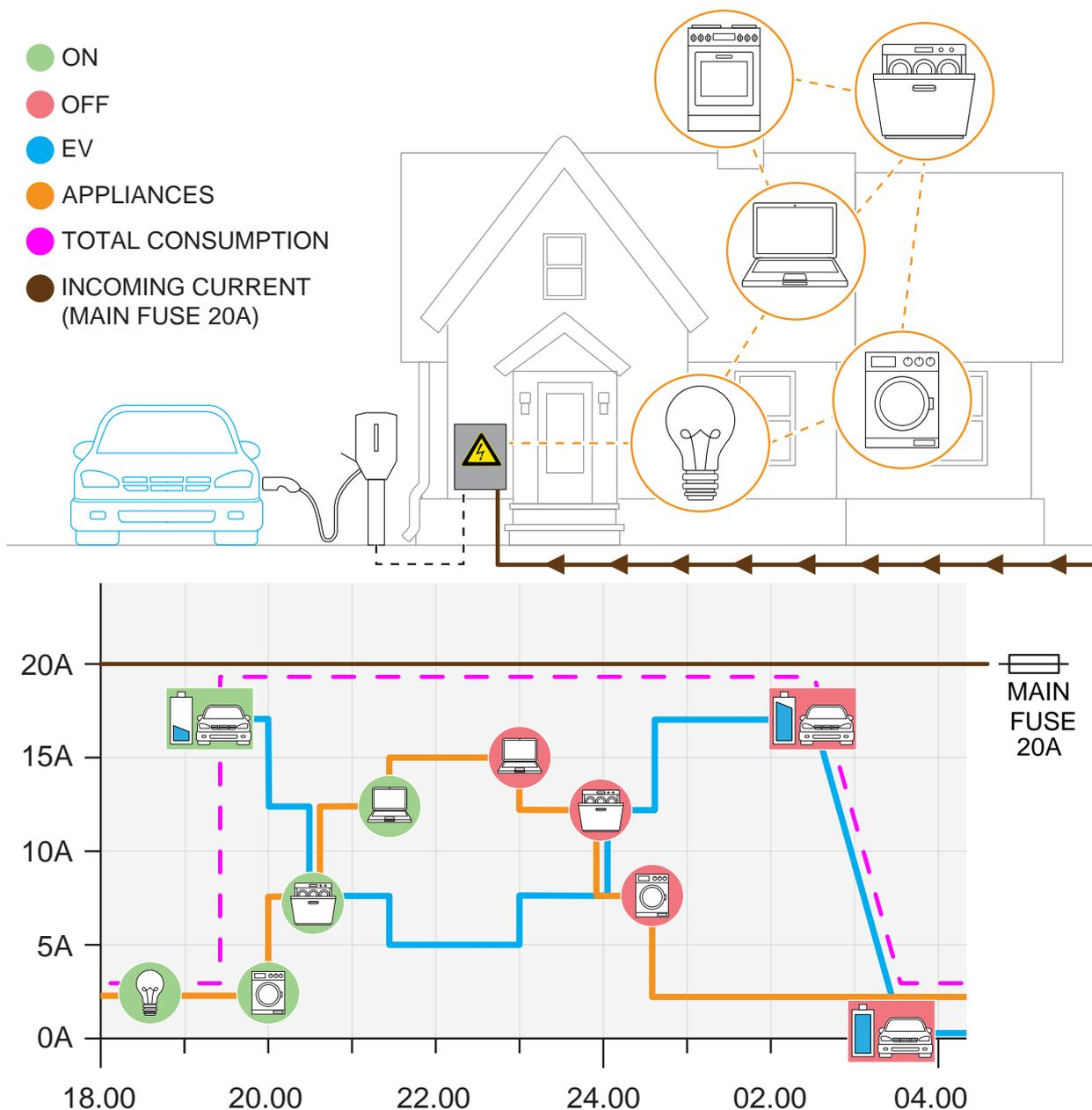
The real current is measured by current transformers or energy meter, and transferred into the system with a load interface. It is possible to define several connection groups as a hierarchy of maximum four levels.
