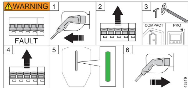
1. If there is an EV connected to the charging station, unplug the Type 2 charging connector. Unlock and remove the front cover of the charging unit, refer to . Do a visual check of all cables and connectors.
