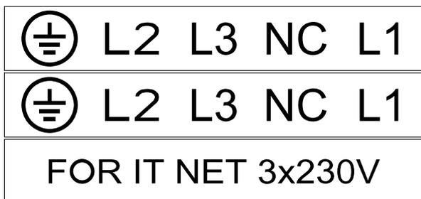
2. Install the new stickers supplied with the installation bracket. Install the new stickers onto the old stickers. Also, attach the "FOR IT NET 3x230V" label on the bracket.
