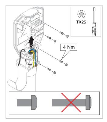
**Note**: Thread the power cable throught the grommet and the ethernet cable through the hole before you attach the screws.
