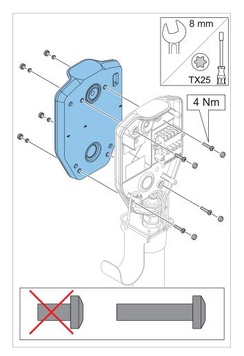
**Note**: Make sure that correct cable grommets are installed in the correct positions on both CS brackets before you attach the CS brackets to the pole mount fixture. Refer to "1. To prepare the CS bracket for installation on the pole mount fixture".
