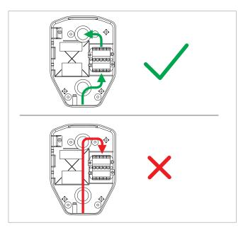
**Note**: No cables or wires may cross the area marked "No Cables".
