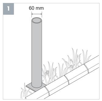
**Note**: Make sure that the pole is attached firmly to the ground.
