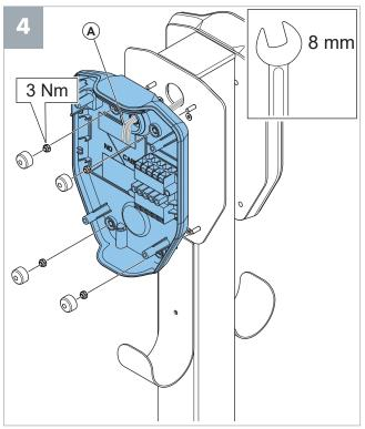
**Note**: Pull out the wires (A) from the first CS units through the cable grommet in the bracket.
