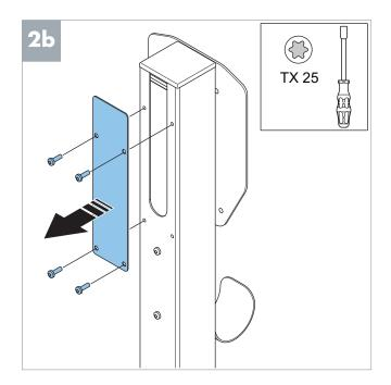
**Note**: Only remove the rear plate if it is necessary when you pull up the cables.
