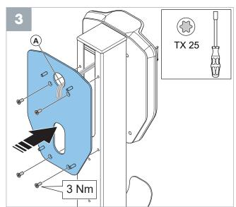
**Note**: Pull out the wires (A) from the first CS units through the top hole of the backplate.
