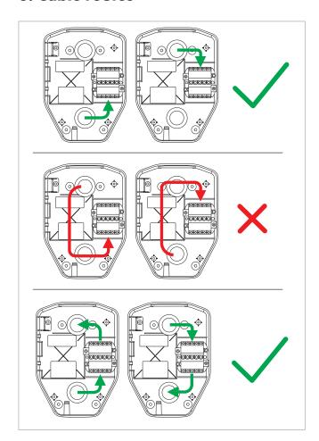
**Note**: No cables or wires may cross the area marked "No Cables".
